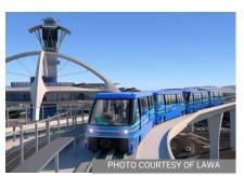
The APM Project will provide an elevated guideway with an at-grade Maintenance and Storage Facility and six stations:
